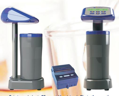
Data transmission to PC or portable printer via Bluetooth connection
