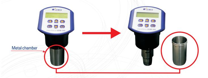
STEP 2: Fill in chamber with sample. Sample volume should be 185±5 ml (48.9±1.3 gal·10<sup>-3</sup>).
