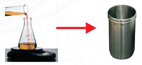
**STEP 3**: Attach metal chamber with sample to the device (Hold chamber on the stable surface!). Place it into the thermostat. Switch ON and start measuring.
